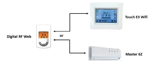
In this system configuration, the parameter 04 in "user menu" becomes an authorization or not of the area to be able to be cooled. The thermostat can't access the "reversible" menu or "automatic" operating mode.
