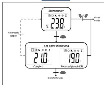
From the screensaver (lighted backlight), by pressing key, temperature set point value is displayed. A second consecutive press can change current mode.
