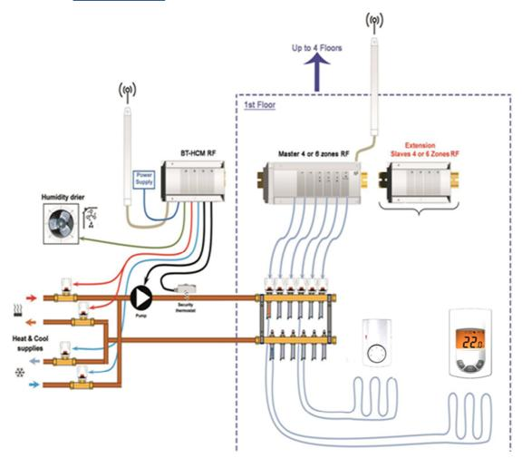
The thermostat is able to communicate with the current products TempCo RF (unidirectional wireless communication "rF.u") and with the products of the new range TempCo E3 web RF (bidirectional wireless communication "rF.b").
