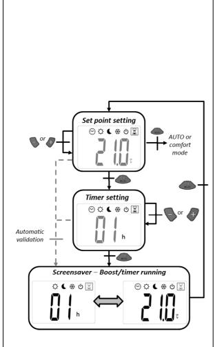
After selecting boost/timer mode (via le AUTO mode or mode selection), by pressing another time switches to the next operating mode (you mustn't have changed temperature set point beforehand, otherwise a second consecutive press is needed).
