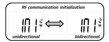
So, when thermostat is in wireless communication initialization step, it sends successively unidirectional and bidirectional pairing frames:
